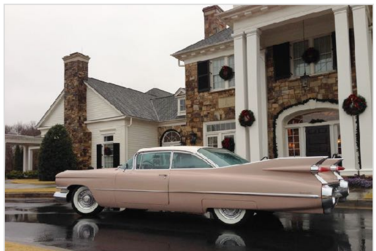
The Series 6200 and Coupe DeVille featured the famous "bubbletop" rear window providing a wide range of visibility to the rear of the car as well as an abundant amount cabin light.
